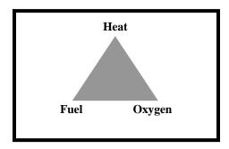
If the sides of the triangle are not allowed to meet – if the triangle does not form, there will be no fire.
